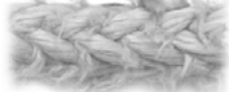
Rope must be replaced
